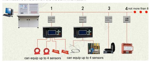
Please note that the independent electrical fire monitoring detector can be connected to the detector loop of the fire alarm controller.
