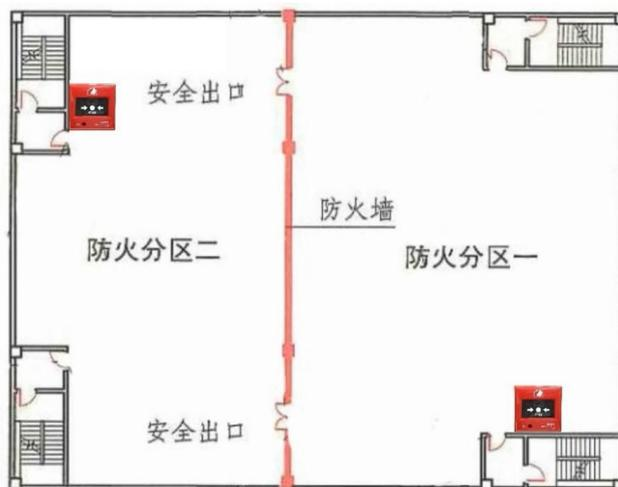
At least one manual fire alarm button shall be provided for each fire zone.
