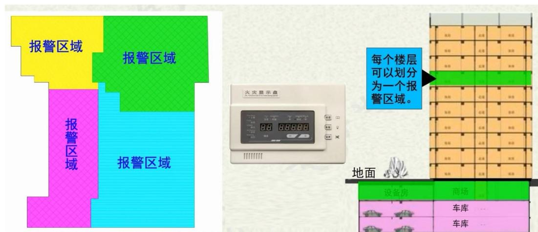
One fire display panel should be set up in each alarm area.
