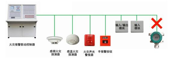
The alarm information and fault information of the combustible gas alarm controller shall be displayed on the graphic display device of the fire control room or on the centrally controlled fire alarm controller.
