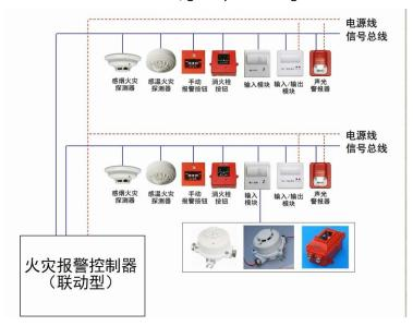
The wire diameter of the bus must meet the impedance requirements and is usually twisted pair, not parallel line, to prevent external electromagnetic interference and cross-talk between lines.
