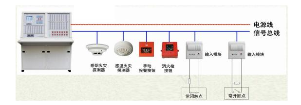
Each module occupies an address point. Address can be set by controller or encoder. A dual input module is a combination of two input modules occupying two address points.
