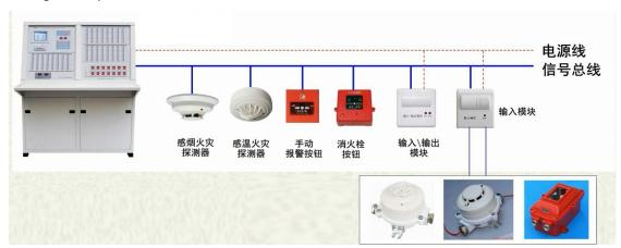
The input module of the non-coded fire detector needs to be connected to the fire power supply. Usually, there is a separate model to distinguish the input module of the equipment signal and facilitate the identification of the system.
