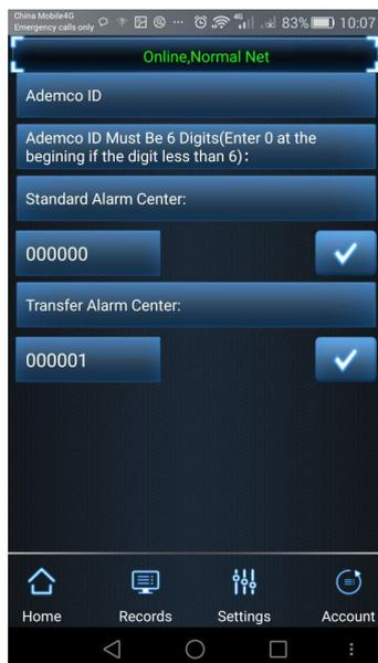
Please note: the Ademco ID of Transfer Alarm Center should be same as the Ademco ID of the software
