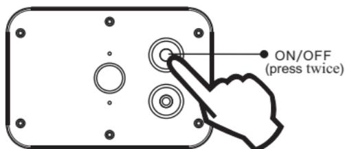
(the light of the ON/OFF button will flash once means the motion sensor was activated and sent the alarm signal)
