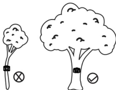
2. Please fix the motion sensor tightly to ensure the position and the direction will not be moved easily by wind.
