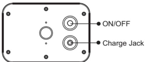
**ON/OFF:** turn on/off the motion sensor
