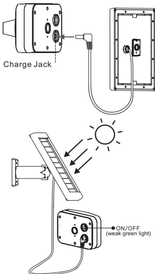
Note: if connection is properly, the ON/OFF button has a weak green light prompt for 30 minutes. Please try your best to make the solar panel face to the sunlight when you install it
