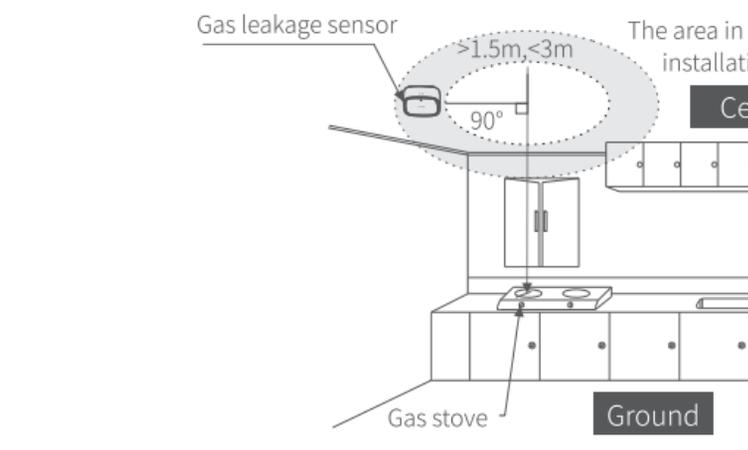
2. Fix the bracket to the wall with screws or 3M tape, then rotate detector into the bracket in clockwise direction. If use 3M tape, please make sure the wall surface firm, smooth and clean, in case of dropping.
