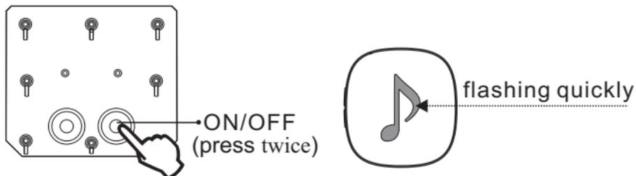
(the light of the ON/OFF button will flash once meaning the motion sensor was activated and sent the wireless signal)
