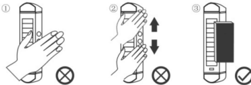
① Infrared light holes are not completely blocked up (Fingers do not completely block up the infrared light holes at the transmitting terminal and the receiving terminal when keeping the transmitting terminal aligned with the receiving terminal).
