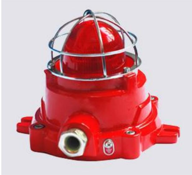
FBSG-YA5801 explosion-proof fire alarm sound and light alarm is non-coding type, suitable for Installation at II C grade, T 6 temperature explosive place. It receiver alarm signal sent from fire alarm control panel and make sound and light warning signal immediately.
