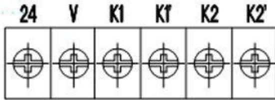
24 V: The Promise of DC24V; K1 K1', : passive output contacts; K2 K2', : passive output contacts
