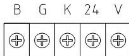
24 V: DC24V (non-polar); BG: normally closed contact; KG: normally open contact
