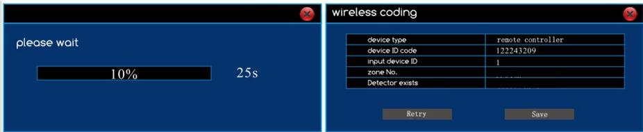
**Related Zone No.:** it is required to associated with 2 neighboring wireless devices in case of preventing from false alarm. Within user set time, trigger two devices, the host will alarm, only trigger one of them, the host device will warn you:[You have entered private place,please exit quickly].
