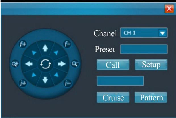
**Note:** The setting of pattern scanning has to be done in PTZ setting. In this screen, it can only be called.
